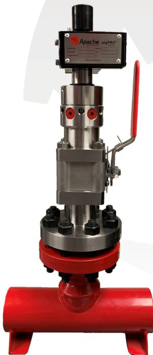
The Series 67 adds safety and servicing options to our existing line intrusive pig passage indicators. Like other available models in the patented pigPRO™ Series, it reliably detects the precise location of a cleaning pig as it travels within the pipeline network. When a pig passes the intruding plunger, it activates the plunger and triggers a visual flag indicator, signaling the pig's location.
